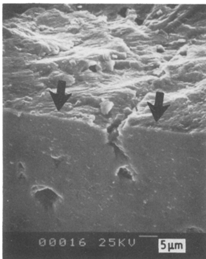
Figure 5 Scanning electron micrograph of a fracture-initiating grain-boundary facet (shown by arrows) in aged Mg-PSZ.
